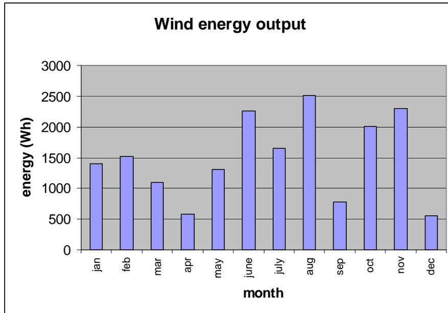
*Figure 16. Potential energy output from the wind system (2001 data) (see Appendix 9 for actual data)*
