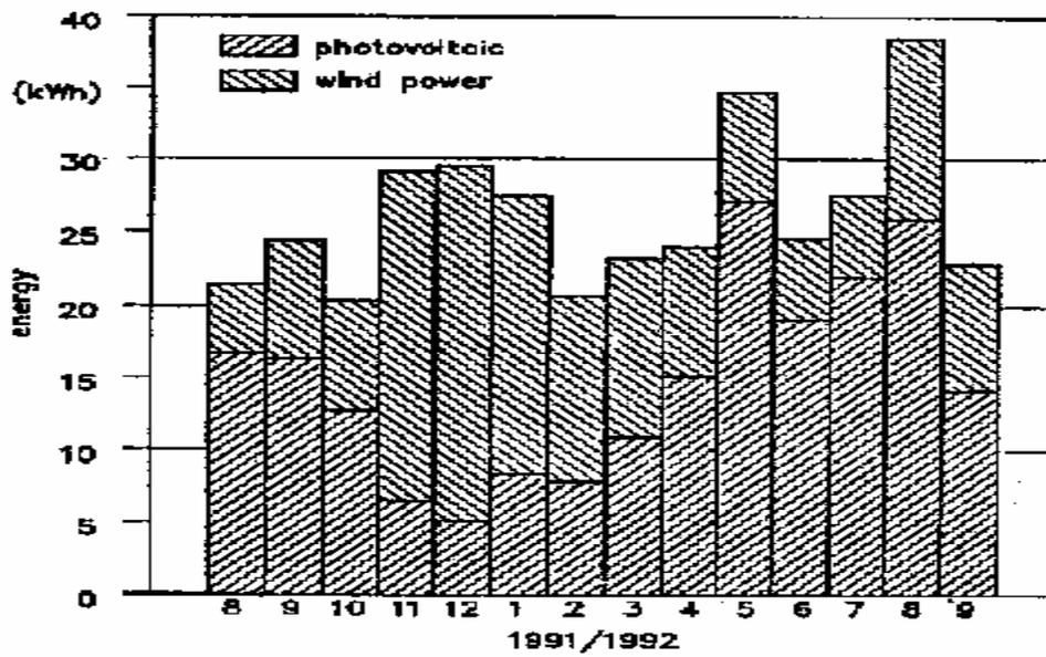
*Figure 1. Energy yield per month of a 220 W PV plant and a 300 W wind driven generator to supply the Daffnerwald Alm in the Bavarian Alps (14)*
