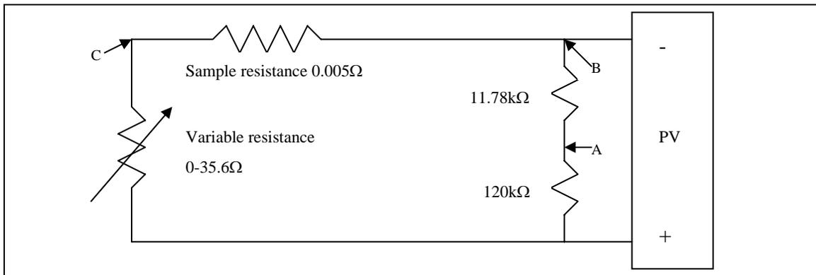
*Figure 2. PV logging system circuit*
