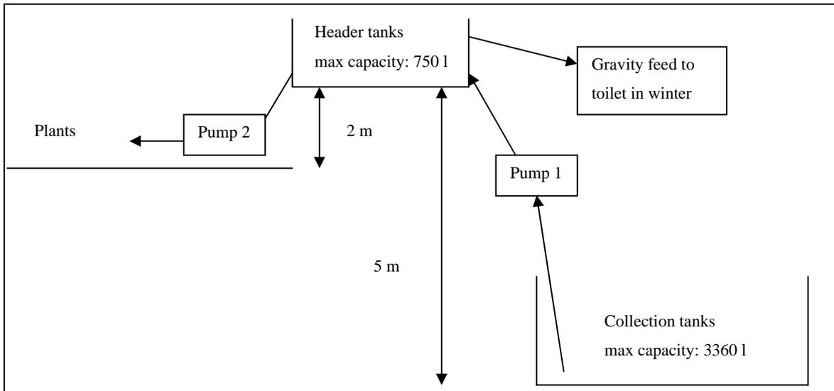
*Figure 18. Pumping system diagram*
