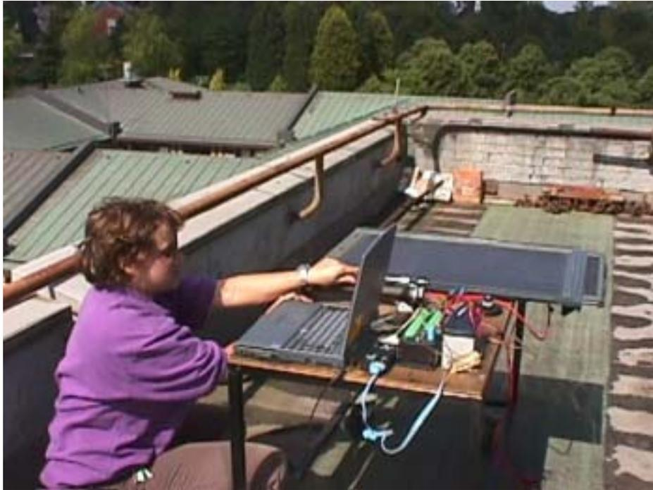
*Figure 3. PV module testing on the Engineering Department roof*
