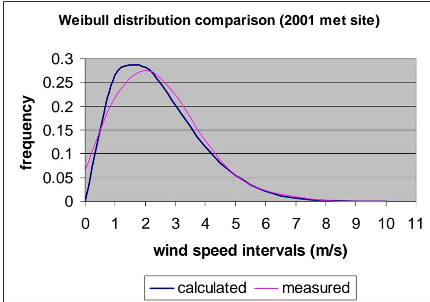
*Figure 10. Measured and calculated wind speed frequency distribution for Reading (10 m hub height)*
