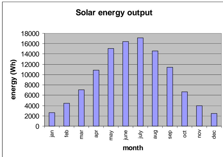
Figure 15. Potential energy output from the solar system (see Appendix 9 for actual data)
