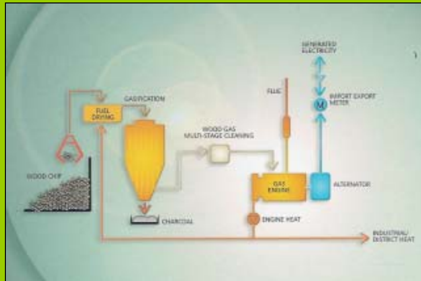
Figure 2b: B9 Wood Gas CHP
