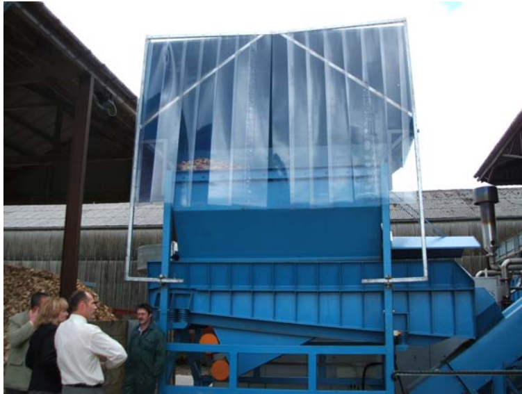
Fuel feed hopper
